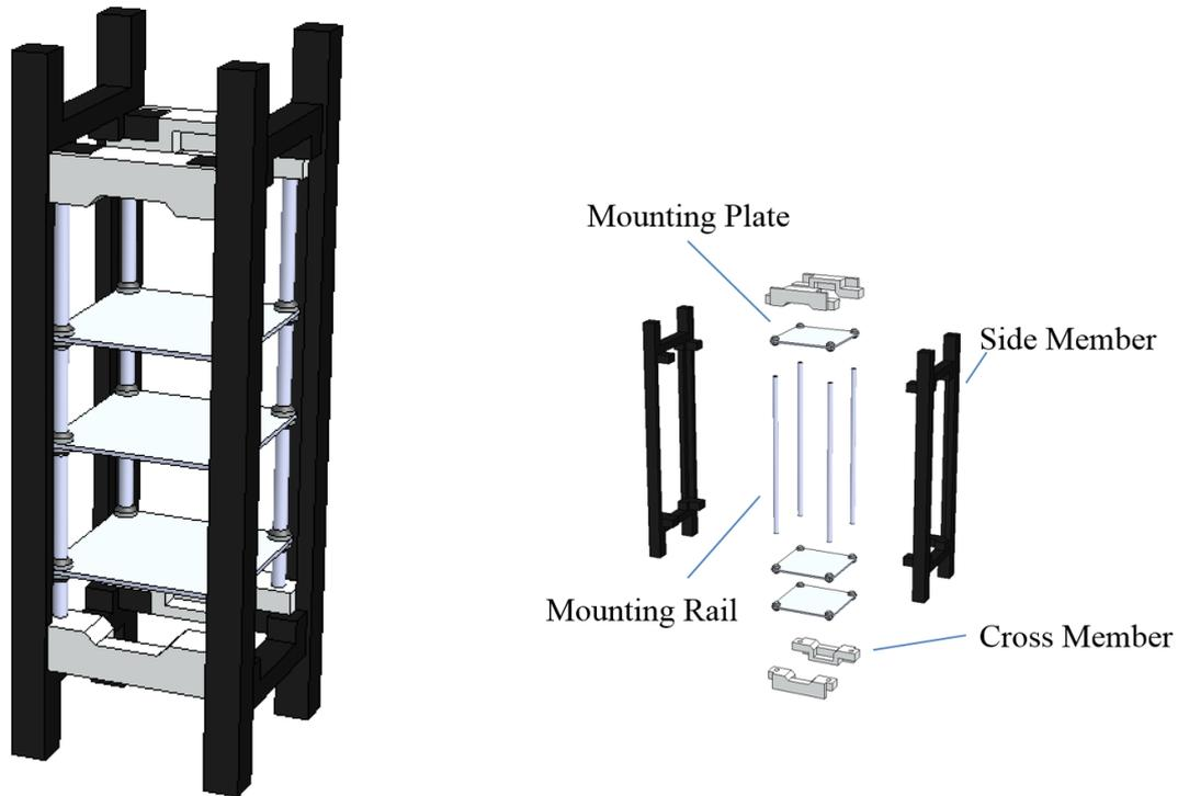
Figure 10: Schematics of main structural components.
