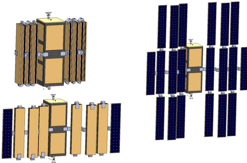
Figure 13: Satellite shown with deployed solar array in three phases
