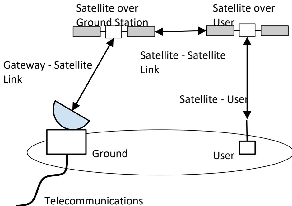
Figure 3: Diagram showing a simplified version of the system, featuring an architecture with Inter-Satellite Links.
