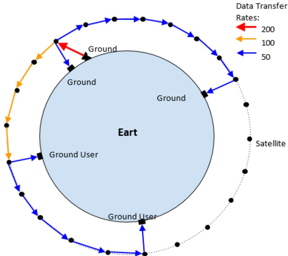
Figure 5: Outward data flow from the Ground Station (connected to terrestrial internet infrastructure) to Ground Users A-D via a single orbital plane of the constellation.
