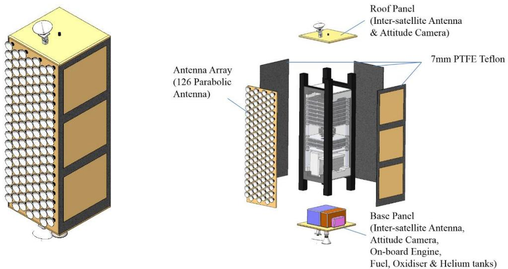
Figure 12: a) CAD of Main Frame assembled b) Exploded view.
