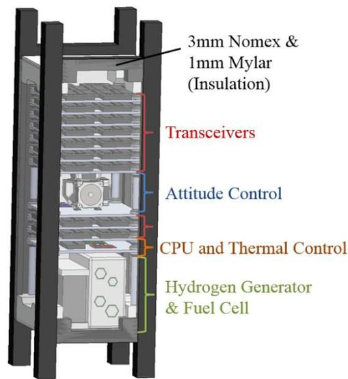
Figure 11: Colour coded CAD of internal components arranged in main frame (inner insulation is shown translucent)
