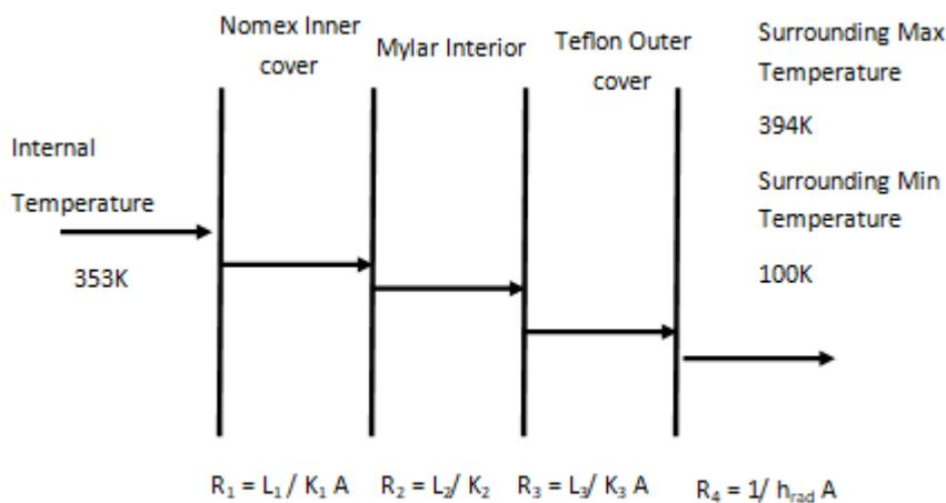
Figure 8: Schematic used to determine insulation requirements.
