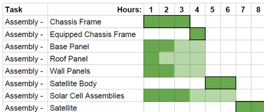
Figure 14: Gantt Chart of the manufacturing process for a single satellite. Dark green indicates the process time and light green any float available. The critical path is highlighted with outlines.
