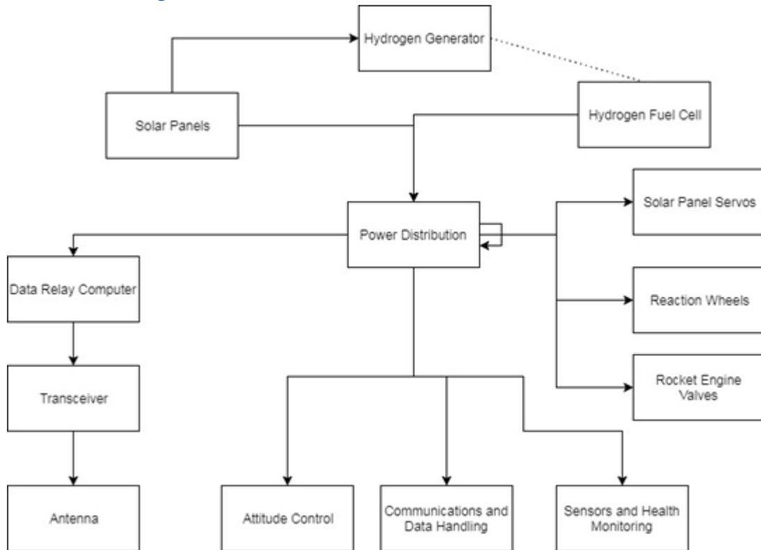
Figure 9: Displays satellites block diagram.
